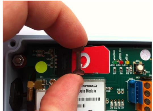
3. **Battery Circuit:** Insert the Bottom board link into pins 2&3 (as shown in **Error! Reference source not found.**) which will connect the RTU's battery. *Note that this link has 3 pins - pins 1&2 are for disconnecting the RTU's battery for long-term storage.*
