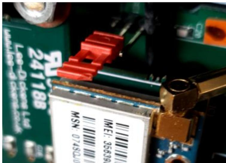
4. **GSM Module Power:** Insert the Top board Battery link – this applies power to the GSM module <sup>4</sup>.
